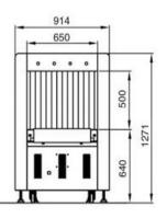
Outer Dimension: 3671mm (L) \*914mm (W) \*1271mm (H) Tunnel Dimension: 500mm (H) \*650mm (W)
